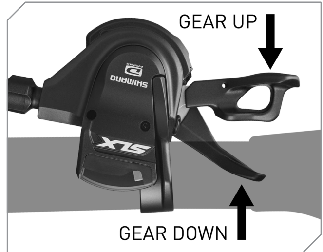
Rapidfire shifter control of the derailleur and Alfine gears
